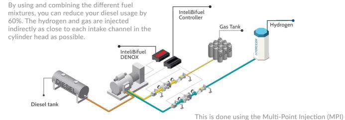
method, which enables precise dosing of the mixture of hydrogen and gas for each cylinder and ensure safe operation of the engine.
