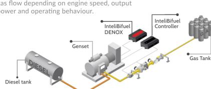
Our simple bi-fuel conversion system modifies your original diesel engine so that it uses gas as the main fuel, which helps to substantially reduce your operating costs without compromising the engine's power output, running time or maintenance schedule.
