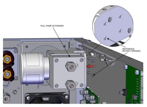
Figure 7–23. Pump Removal, Keyway
