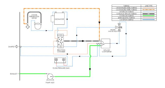
Figure 1–2. 42iQLS Flow Schematic
