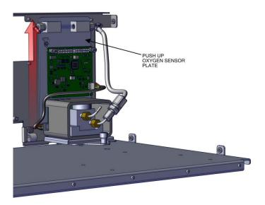
Figure 7–58. Oxygen Sensor Removal pt 3
