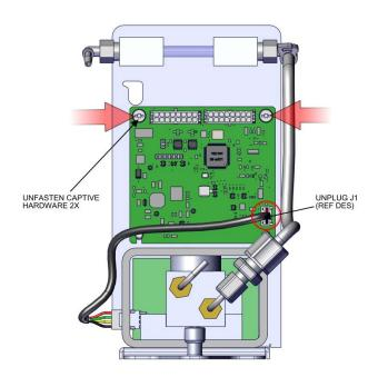
Figure 7-60. Replacing the Oxygen Sensor DMC Board
