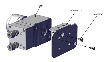
Figure 7–24. Pump replacing, Unfasten Screws
