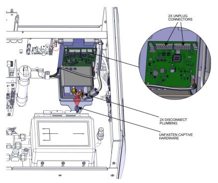
Figure 7-56. Oxygen Sensor Removal pt 1
