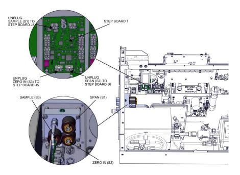
Figure 7–51. Replacing the Manifold pt 1
