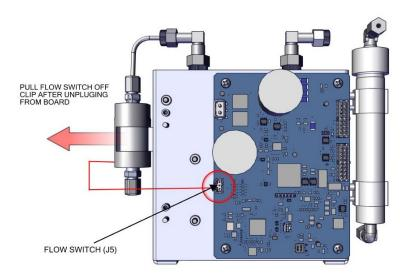
Figure 7–49. Flow Switch Remove
