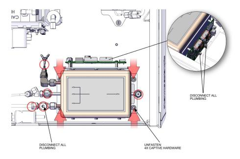
Figure 7–41. Converter DMC Assembly Remove
