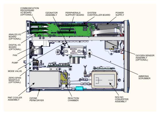
Figure 7-2. 42iQLS Component Layout Top View
