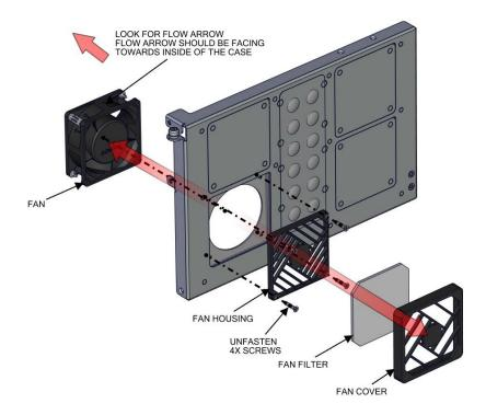
Figure 7–8. Replacing the Fan
