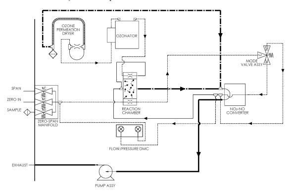
Figure 9–9. Flow Diagram, Zero/Span Option
