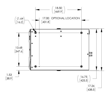
Figure 1-4. Bench Mount Assembly (dimensions in inches [mm])
