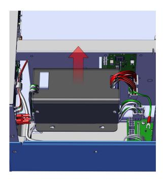
Figure 7–26. Replacing Power Supply
