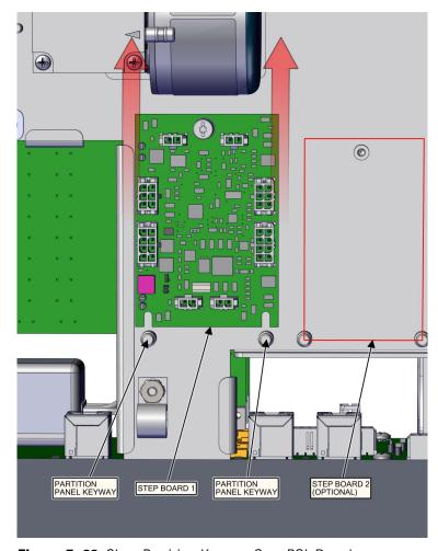
Figure 7–28. Clear Partition Keyway Step POL Board
