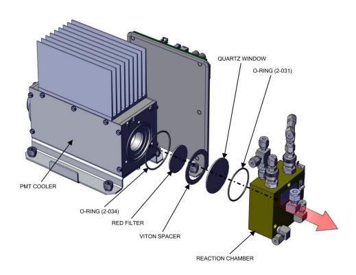
Figure 7–36. Photo Reaction Chamber Cleaning, Window
