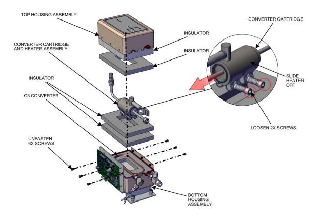
Figure 7–43. Converter Assembly Replace Heater
