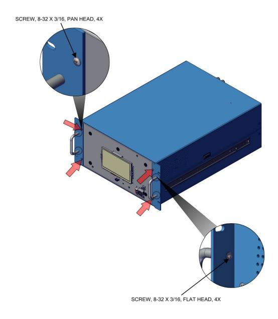
Figure 2–4. Installing Ears and Handles
