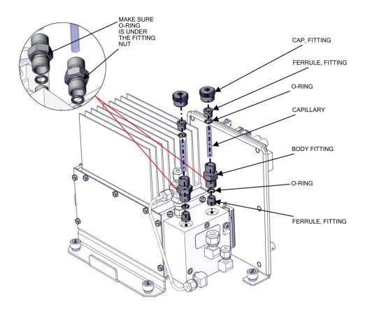
**Figure 5–1.** Inspecting and Replacing the Capillaries
