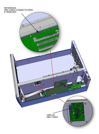
Figure 7–10. Unplugging the DMC Cable
