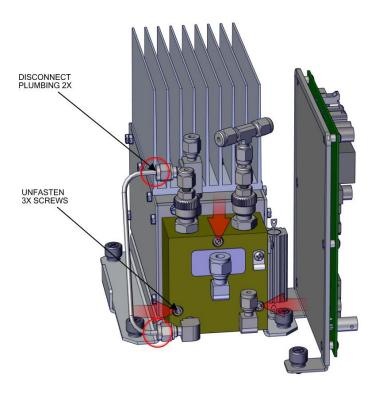
Figure 7–35. Photo Reaction Chamber Cleaning, Hardware
