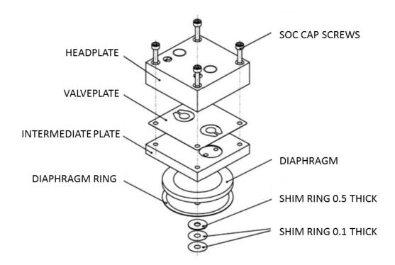
Figure 5–3. Pump Rebuilding
