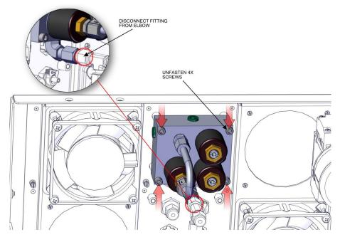
Figure 7–53. Replacing the Manifold pt 3
