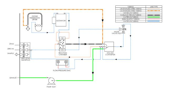
Figure 1–3. 42iQLS Flow Schematic with Zero Span
