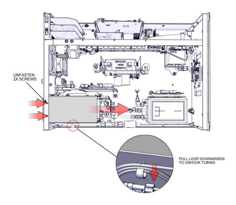
Figure 7–31. Remove PMT Cooler Shroud
