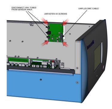
Figure 7–21. Flow Pressure Board, Screws
