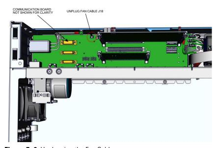
Figure 7–9. Unplugging the Fan Cable
