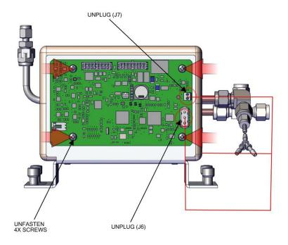
Figure 7–42. Converter Assembly Remove bd
