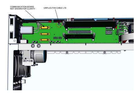
Figure 7–7. Unplugging the Fan Cable
