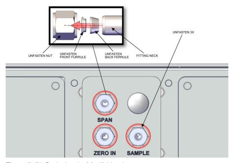
Figure 7–52. Replacing the Manifold pt 2
