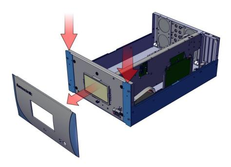
Figure 2–3. Removing the Front Panel
