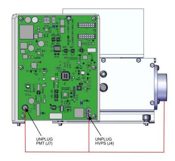
Figure 7–37. PMT Tube Replace-Elec-Pt1
