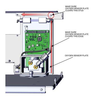
Figure 7–57. Oxygen Sensor Removal pt 2
