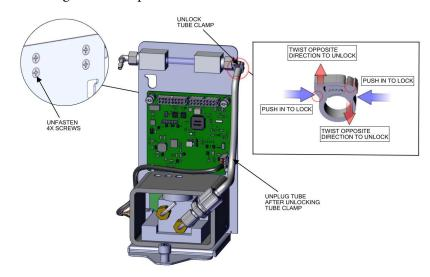
Figure 7–62. Replacing the Oxygen Sensor Capillary
