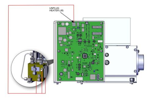
Figure 7–34. Photo Reaction Chamber Cleaning, Electrical
