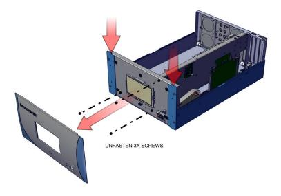
Figure 7–11. Unfasten Hardware Front for Measurement Side Removal
