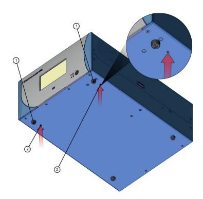
Figure 2–2. Installing Feet
