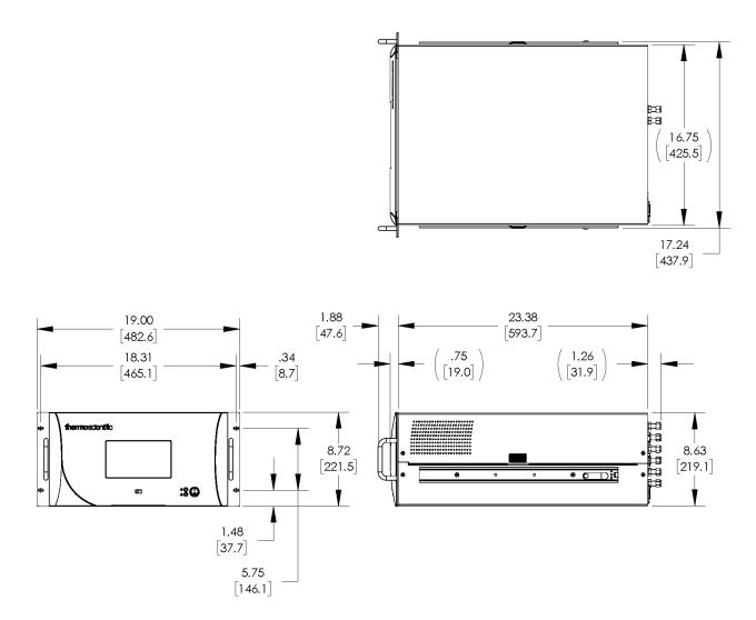
Figure 1–5. Rack Mount Assembly (dimensions in inches [mm])
