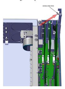
Figure 7–15. I/O Replacement, Arm
