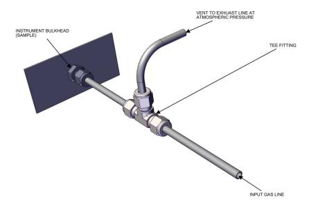
Figure 2–6. Atmospheric Dump Bypass Plumbing
