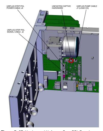
Figure 7-27. Unplug and Unfasten Step POL Board
