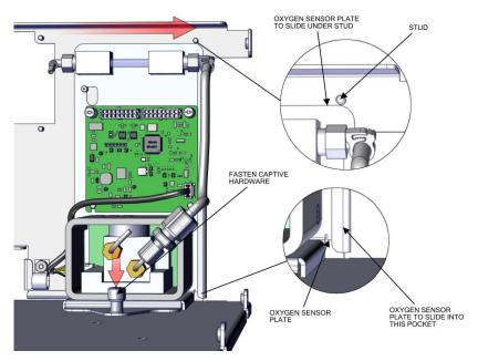
Figure 7–66. Oxygen Sensor DMC install pt 2
