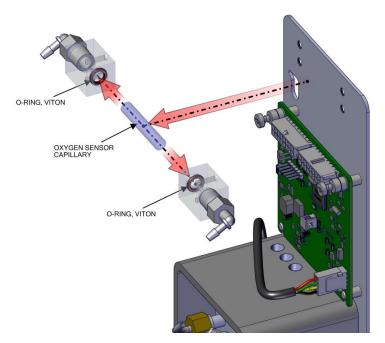
Figure 7–63. Replacing the Capillary pt 2
