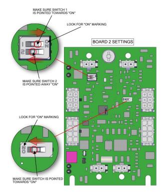
Figure 7–30. Step POL Board 2 Switch Settings
