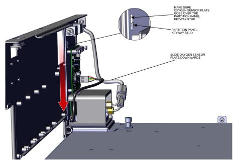
Figure 7–65. Installing the Oxygen Sensor DMC
