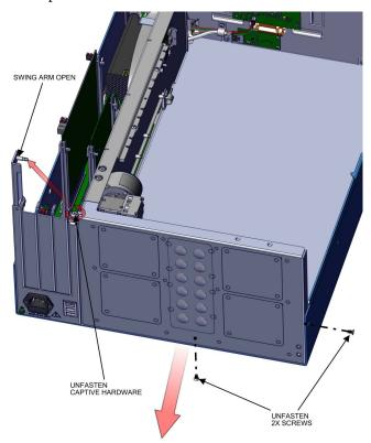
Figure 7–12. Unfasten Hardware Rear for Measurement Side Removal
