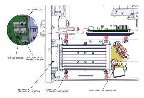
Figure 7–32. Remove DMC PMT Cooler
