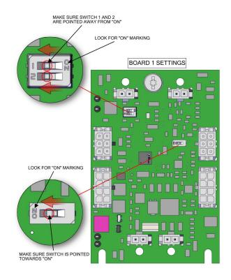
Figure 7–29. Step POL Board 1 Switch Settings
