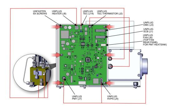
Figure 7–33. Remove PMT Cooler Board
