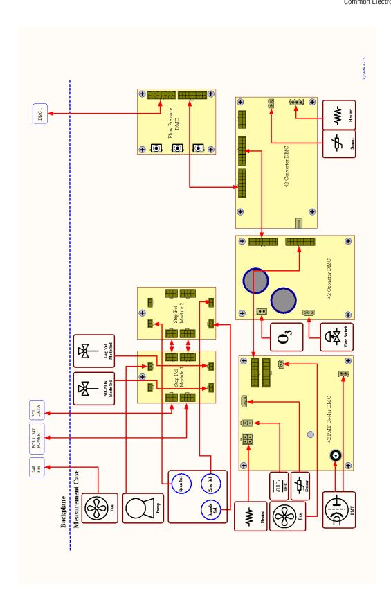
Figure 8–2. 42iQLS System Interconnect Diagram
