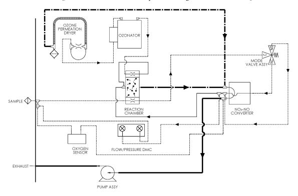
Figure 9–10. 42iQLS Flow Schematic with Internal O<sub>2</sub> Sensor
