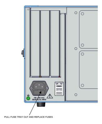
Figure 7–4. Replacing the Fuses
