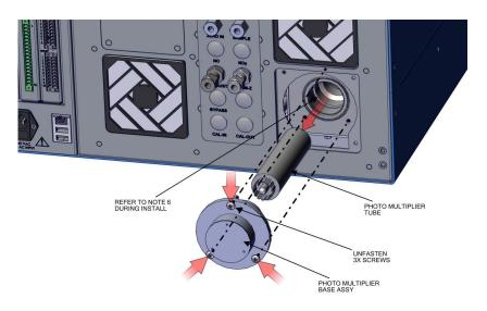
Figure 7–40. PMT Tube Replace-Screws
