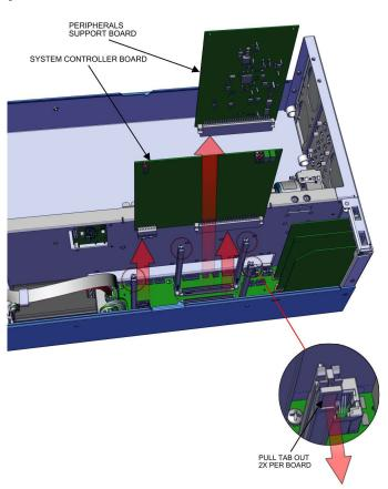
Figure 7–19. Replacing the Peripherals Support Board
