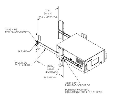
Figure 1–6. Rack Mount Requirements
