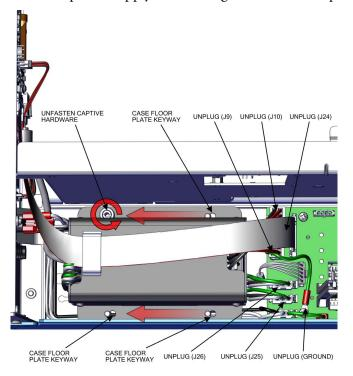
Figure 7–25. Removing Power Supply
