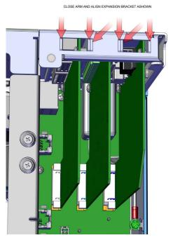
Figure 7–18. I/O Replacement, Close Arm Alignment
