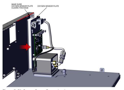
Figure 7–59. Oxygen Sensor Removal pt 4
