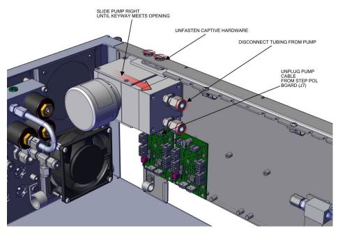
Figure 7–22. Remove Pump, Disconnect and Unfasten
