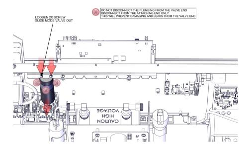
Figure 7-55. Mode-Lag-Perm Hardware, Plumbing
