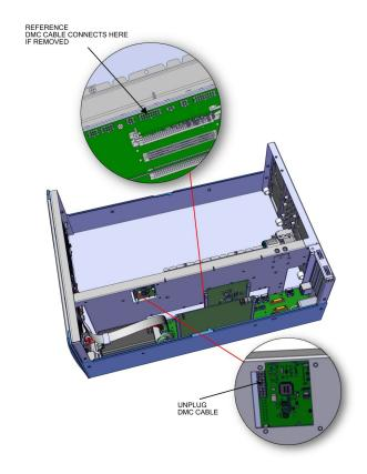
Figure 7–20. Flow Pressure Board, Disconnect DMC Cable
