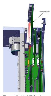
Figure 7–16. I/O Replacement, Remove Board
