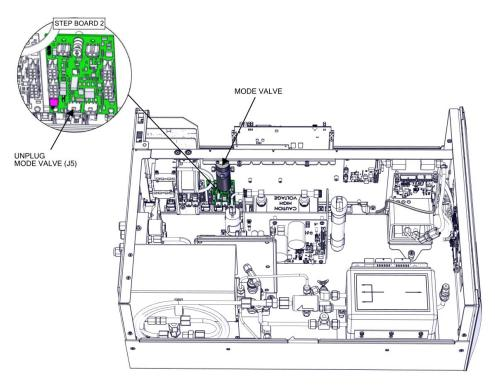
Figure 7–54. Mode-Lag-Perm Electrical Connection
