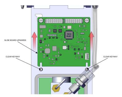
Figure 7–61. Replacing the Oxygen Sensor DMC Board pt 2
