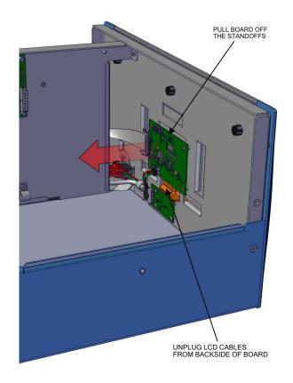
Figure 7–14. Remove Electrical Cables from LCD
