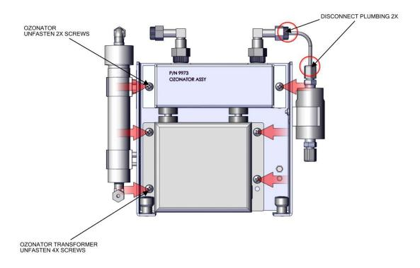
Figure 7-47. Replace Transformer
