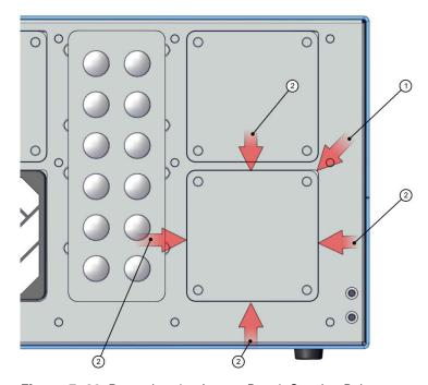
Figure 7–38. Removing the Access Panel, Starting Point
