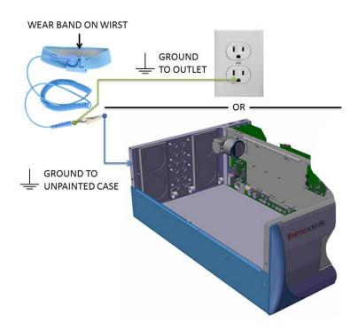
Figure 7–1. Properly Grounded Antistatic Wrist Strap
