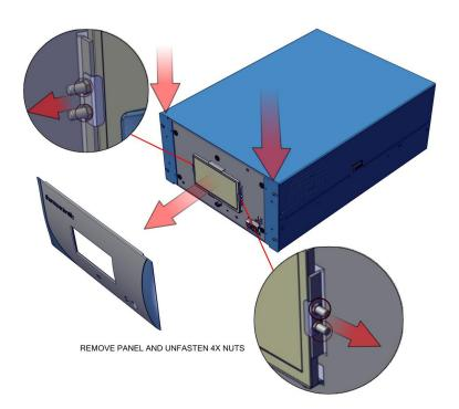
Figure 7–13. Replacing the LCD Module
