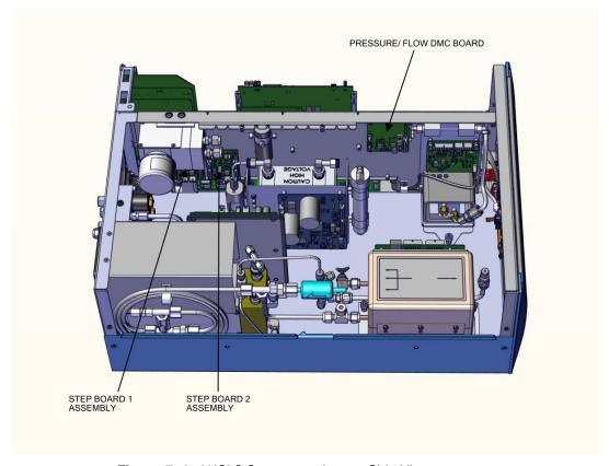
Figure 7–3. 42iQLS Component Layout Side View
