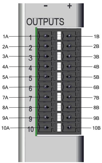
Figure 9–7. Digital Relay Switches
