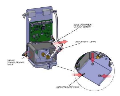
Figure 7-64. Replacing the Oxygen Sensor
