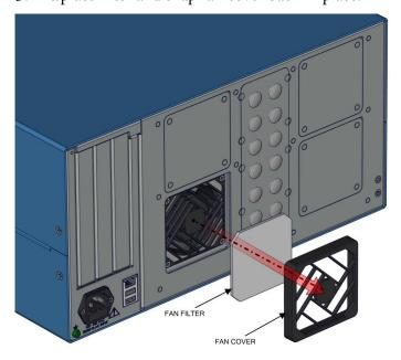
Figure 7–6. Removing the Fan Cover
