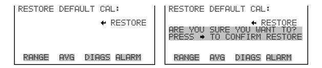
**Calibration Menu** The Calibration menu is used to automatically set the zero background and the span coefficient. The zero/span check menu item is visible only if the zero/span valve option is installed.
