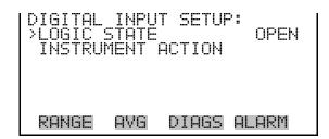
**Instrument Action** The Instrument Action submenu allows the user to choose the instrument action that is assigned to the selected digital input. The zero and span modes are only present if the zero/span valve option is installed.
