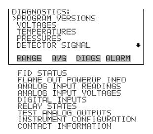
**Program Versions** The Program Versions screen (read only) shows the version numbers of the programs installed. Prior to contacting the factory with any questions regarding the instrument, please note the product model name (51*i*HT or 51*i*LT) and the program version numbers.
