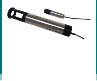
The PD-Mini data logger is a compact device for level monitoring of groundwater wells. Besides water level it acquires air pressure, temperature and battery voltage. The recorded data can be downloaded by a 433-MHz radio USB adapter (available as accessory) and a support software that exports measurement data as Excel files.
