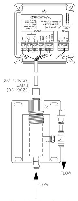
Figure 8 - Loop-Power Connection
