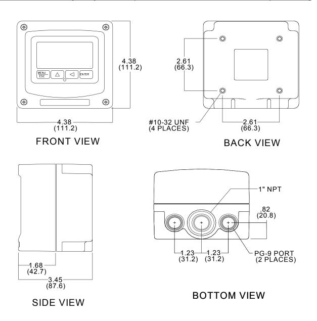
Figure 2 - Q45 Enclosure Dimensions
