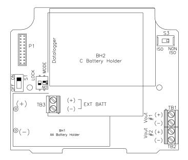
Figure 9 - External Power Board
