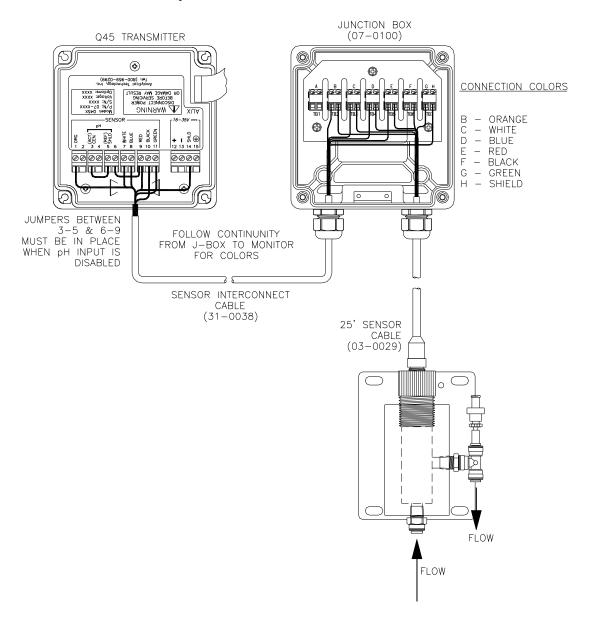
Figure 11 Junction Box Interconnect Wiring
