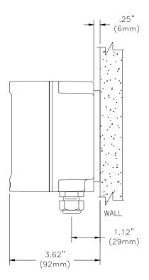
Figure 4 - Wall Mount Diagram
