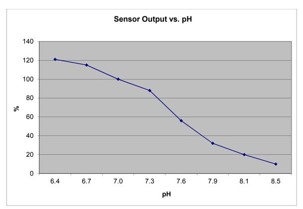
Figure 18 - Typical Chlorine Response to Change in pH
