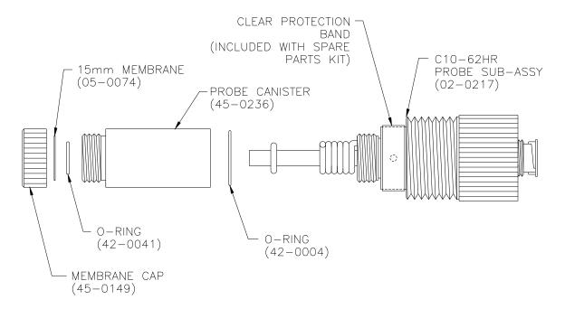
Figure 13 Chlorine Sensor Assembly
