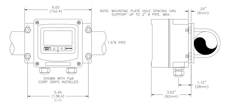
Figure 5 - Pipe Mount Diagram
