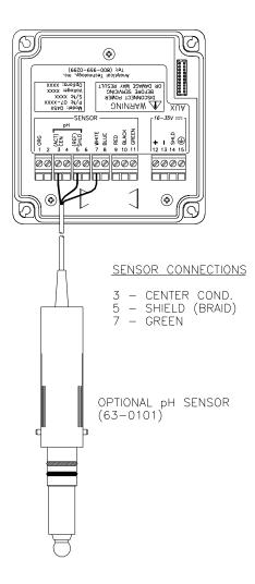
Figure 12 - Optional pH Sensor Connection
