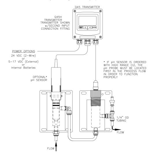
Figure 1 - Typical Chlorine Monitoring System
