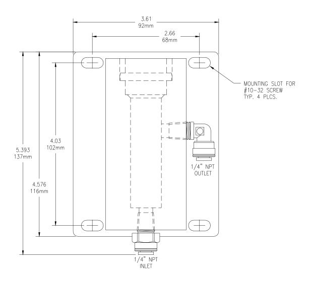
Figure 7 - Sealed pH Sensor Flowcell
