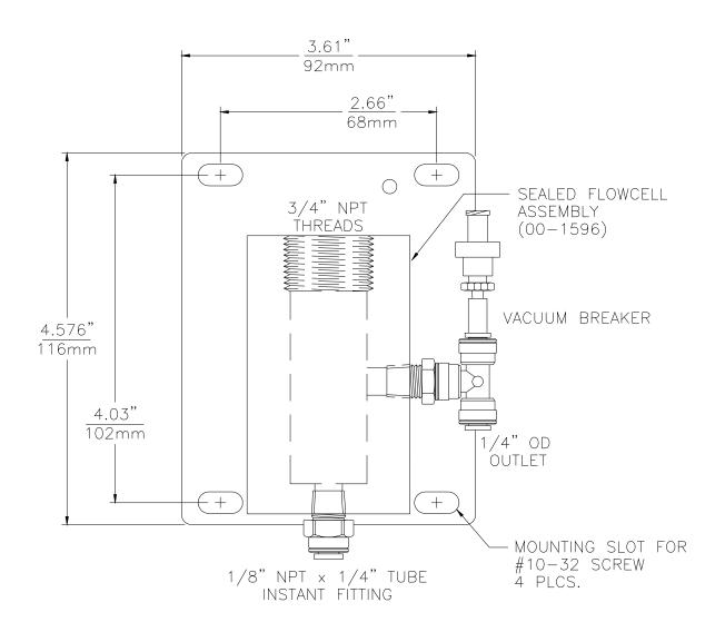
Figure 6 - Sealed High Range Sensor Flowcell
