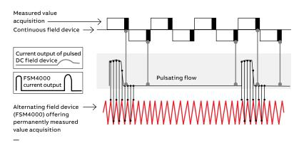
In offering nearly uninterrupted sampling of the flow signal, AC field technology is extremely well suited to measure pulsating flow, generated by piston pumps, diaphragm pumps or hose pumps. Flowmeters working with DC field technology can only acquire pulsating flow data intermittently.
