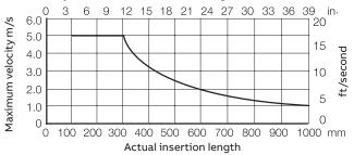
Figure 8 Maximum allowable velocity for different insertion lengths
