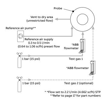
AutoCal with test gas(es) and restrictors
