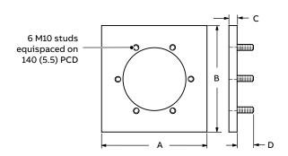
Standard mounting plate for 1.0 to 4 m (3.3 to 13.1 ft) probes – part No. AZ200 795
