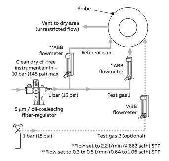
AutoCal with air supply and restrictors
