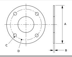
4-hole probe flange types and dimensions
