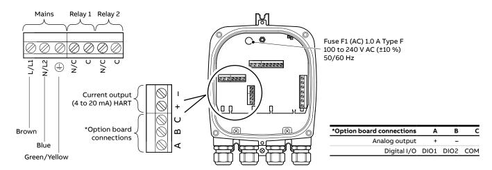
Remote transmitter – power supply and output connections
