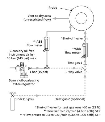
Non-AutoCal with air supply and restrictors
