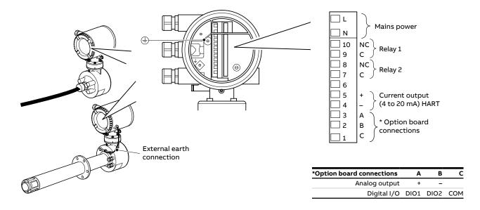
Integral transmitter - power supply and output connections
