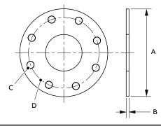
8-hole probe flange types and dimensions
