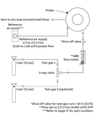
Non-AutoCal with test gas(es) and restrictors
